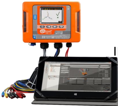
POWER QUALITY METER
