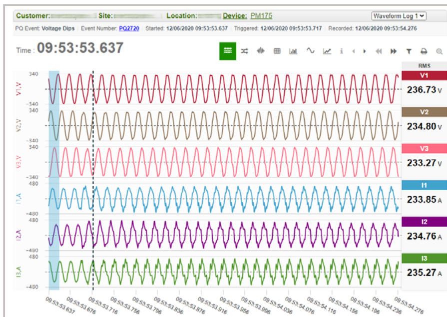
Figure 3: Voltage Dip, viewed on SATEC's Expertpower software
